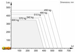
The KR 600 R2830 is designed for a rated payload of 600 kg in order to optimize the dynamic performance of the robot. The maximum payload of 729 kg applies only if the position of the center of mass is 0 mm and a supplementary load optimized for the load case is mounted. The specific load case must be verified using KUKA.Load or KUKA Compose. For further consultation, please contact KUKA Support.
