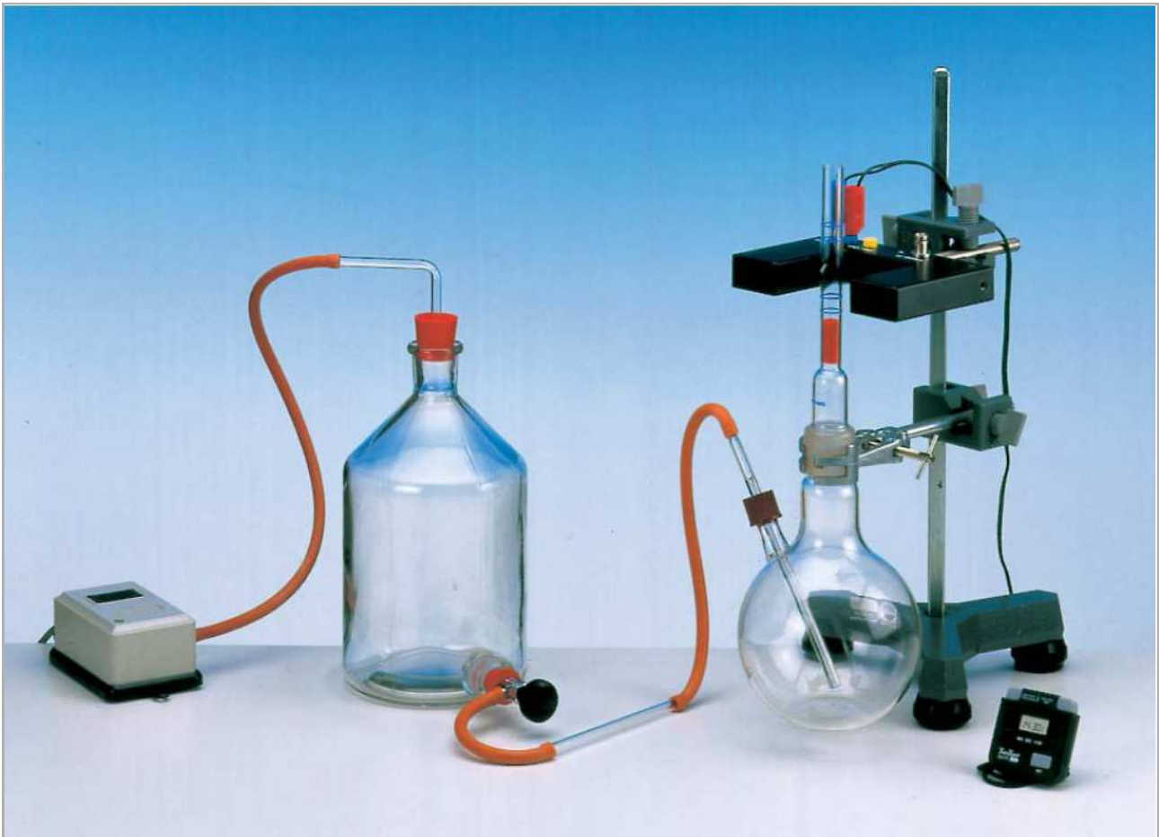
Fig. 1: Experimental set-up: Adiabatic coefficient of gases – Flammersfeld oscillator.
