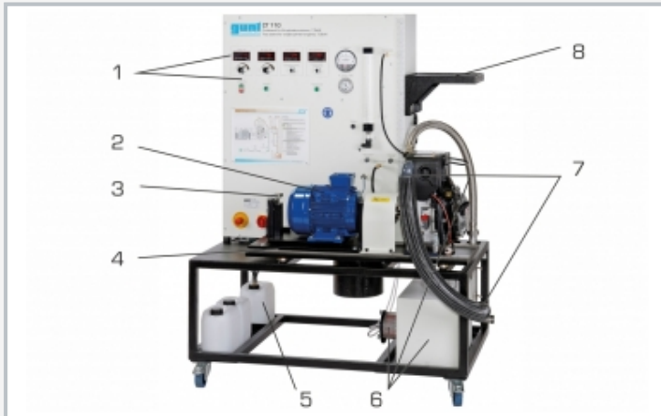
1 display and control panel, 2 asynchronous motor, 3 force sensor (torque), 4 base plate, 5 fuel tank with pump, 6 stabilisation tank with air filter and air hose, 7 exhaust gas connection, 8 shelf, e.g. for CT 100.13
