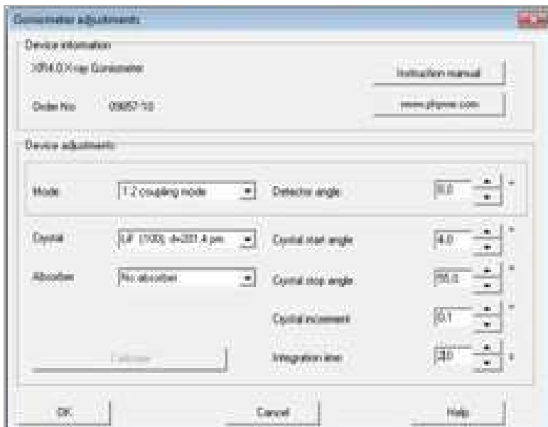
Fig 6: Settings of the goniometer (LiF crystal)
