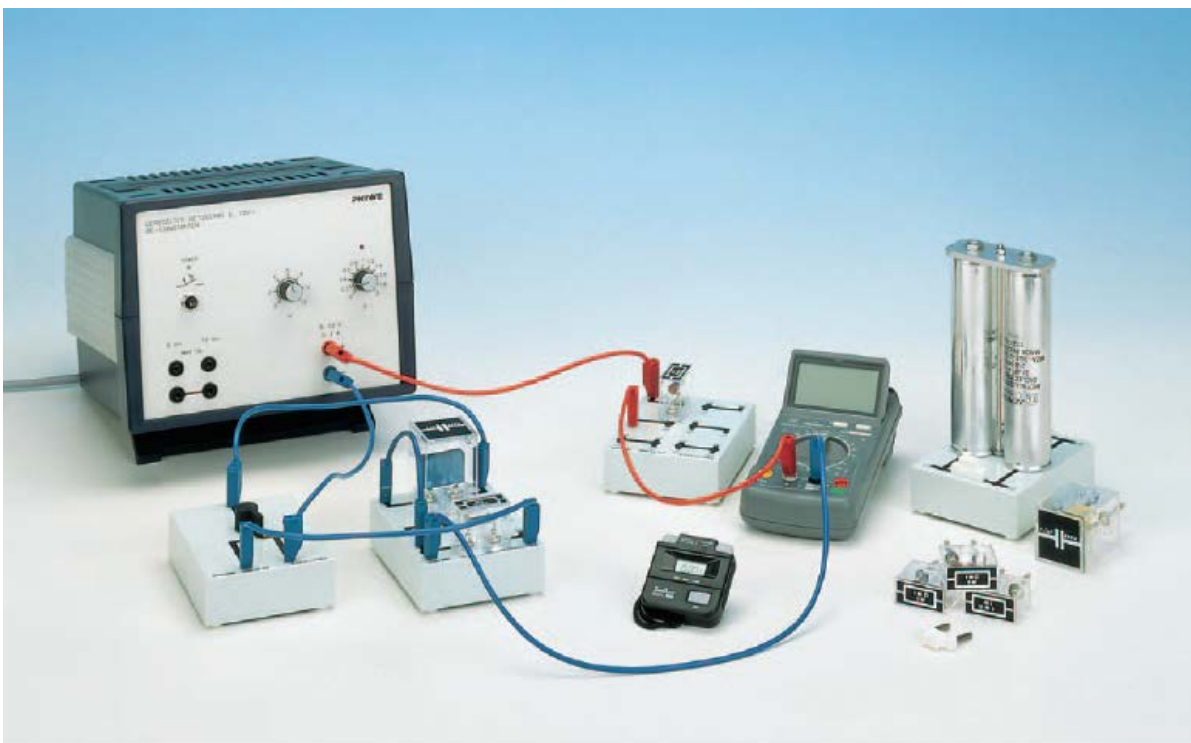
Fig. 1: Experimental set-up for measuring the current when a capacitor is being charged.
