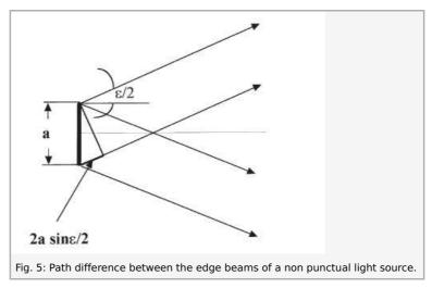
$(\lambda = wavelength; a = extension of the light source; \varepsilon = angle of aperture of the conical light beam used to generate interference; g = distances between the slit centres of the double slit; d = slit width of the double slit; L = distance between light source and double slit).$
