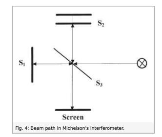
Shifting the mirror  $S_2$  by a distance D and observing the aberration of n dark zones, the wavelength is obtained from the following equation:
