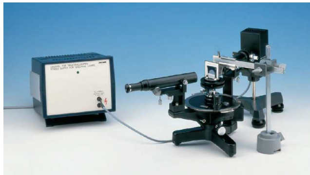
Fig. 3: Experimental set-up with vernier used auxiliary slit to determine the resolving power.
