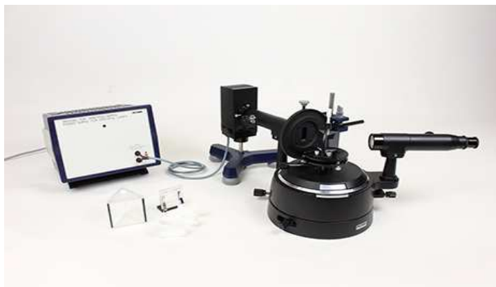
Fig. 1: Experimental set-up for determining dispersion in liquids.
