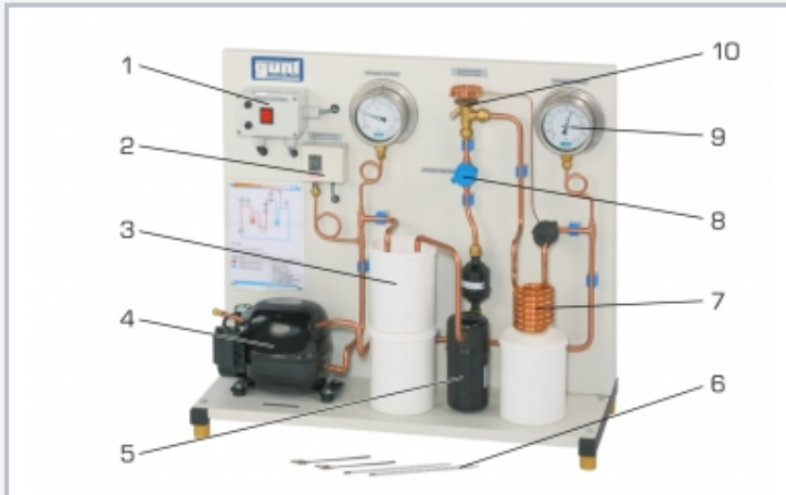
1 main switch, 2 pressure switch, 3 evaporator with water tank, 4 compressor, 5 receiver, 6 thermometer, 7 condenser, 8 sight glass (refrigerant), 9 manometer, 10 expansion valve
