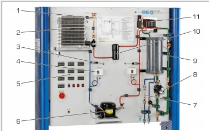
1 expansion valve, 2 evaporator with fan, 3 pressure sensor, 4 pressure switch, 5 displays and controls, 6 compressor, 7 cooling water flow meter, 8 pump, 9 hot water tank, 10 receiver, 11 cocondenser
