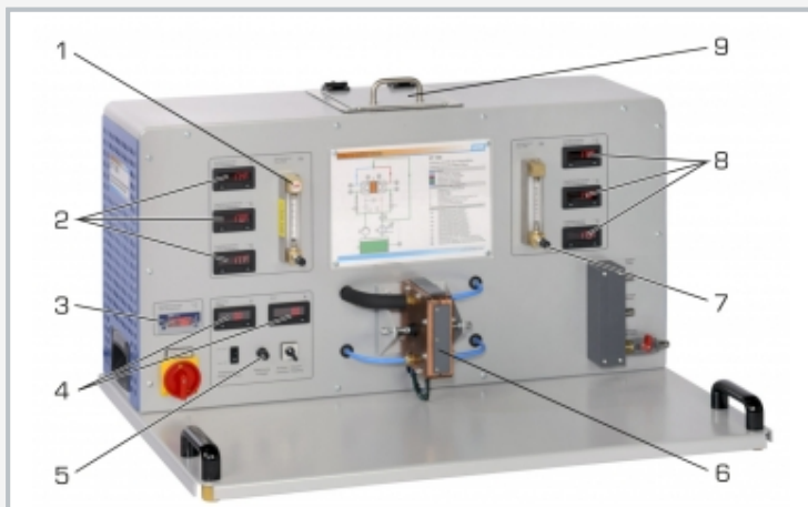
1 cold water flow meter, 2 temperature displays cold side, 3 water tank temperature controller, 4 voltage and current displays, 5 adjustment of the electrical power, 6 Peltier element with heat exchangers, 7 hot water flow meter, 8 temperature displays hot side, 9 water tank cover
