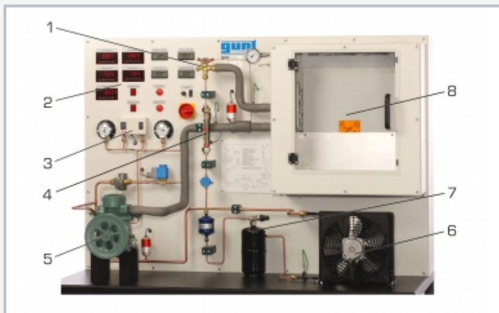
1 expansion valve, 2 displays and controls, 3 pressure switch, 4 flow meter, 5 compressor, 6 condenser, 7 receiver, 8 refrigeration chamber
