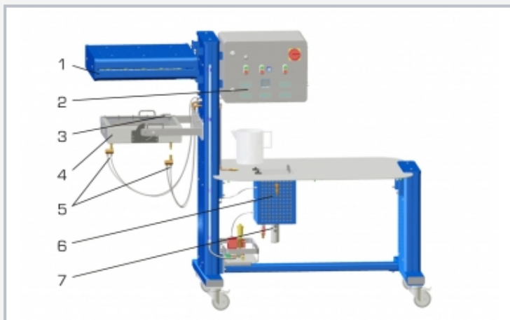
1 lighting unit, 2 control cabinet, 3 illuminance sensor, 4 flat collector with spacing and tilt adjustment, 5 temperature sensor, 6 storage tank, 7 electrical auxiliary heater
