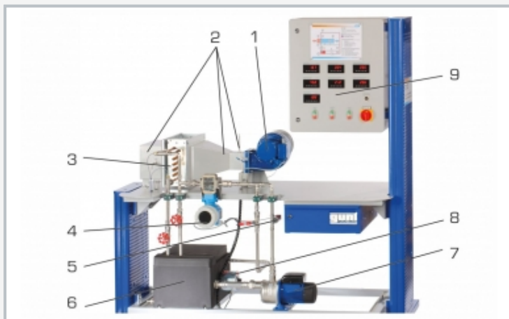
1 fan, 2 air duct with temperature measuring points, 3 heat exchanger, 4 flow meter, 5 pressure sensor, 6 water tank, 7 pump, 8 heater with thermostat, 9 displays and controls
