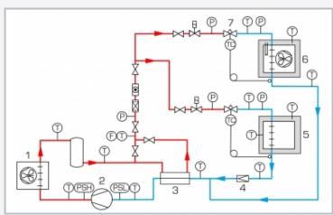
1 condenser, 2 compressor, 3 heat exchanger, 4 evaporation pressure controller, 5 refrigeration chamber, 6 freezing chamber with defrost heater 7 expansion valve; T temperature, P pressure, F flow rate, PSH, PSL pressure switch
