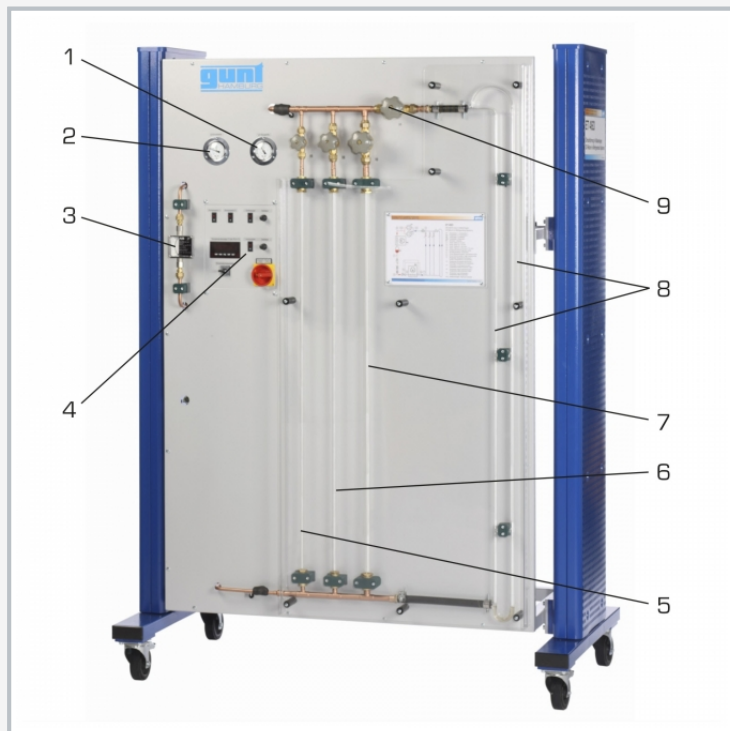
1 manometer delivery side, 2 manometer intake side, 3 flow meter, 4 display and control elements, 5 rising pipe d=6mm, 6 rising pipe d=10mm, 7 rising pipe d=14,4mm, 8 double rising pipe, 9 valve for rising pipe selection
