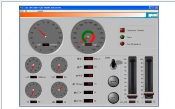
Software screenshot: control panel of a two-shaft gas turbine
