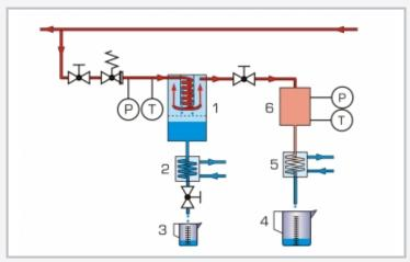
1 water separator with cyclone, 2 cooler, 3 measuring cup for separated water, 4 measuring beaker for liquefied vapour, 5 condenser, 6 tank for depressurising the vapour, red: wet steam, orange: depressurised steam, blue: water, P pressure, T temperature
