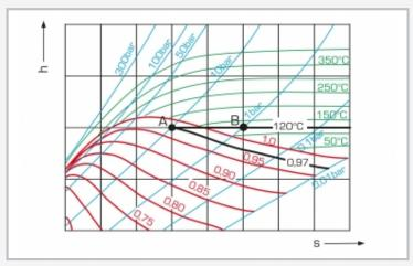
h-s diagram; h enthalpy, s entropy; red: vapour content, green: temperature, blue: pressure; black: example of measuring result: A steam at 10bar, B steam after adiabatic depressurisation at 1bar, vapour content 0,97
