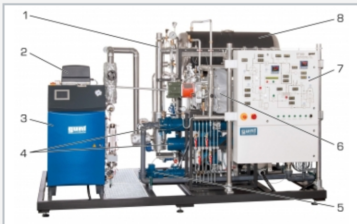
1 superheater, 2 burner, 3 boiler, 4 condenser, 5 condensate pump, 6 turbine, 7 displays and controls, 8 feedwater tank with feedwater treatment
