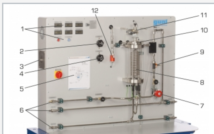
1 displays and controls, 2 valve for sealing steam, 3 steam connection, 4 valve for steam inlet, 5 process schematic, 6 water connections, 7 pressure sensor for condensate measurement, 8 condenser with coil, 9 cooling water flow rate sensor, 10 turbine, 11 eddy current brake, 12 pressure sensor
