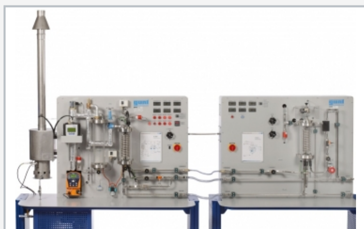
Left: ET 850 Steam Generator and right: ET 851 Axial Steam Turbine; assembled ready for operation, together both units form a complete steam power plant
