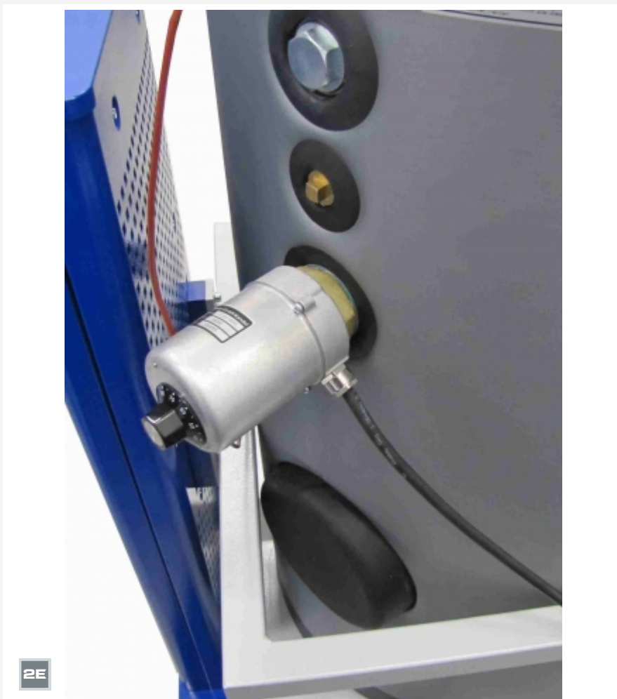
HL 320.02 heater installed in the bivalent storage tank of HL 320.05
