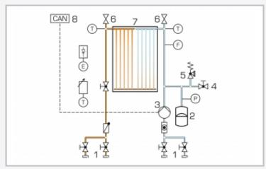
1 connections for heat transfer pipes with shut-off valves and quick-release coupling, 2 diaphragm expansion vessel, 3 pump, 4 fill valve, 5 pressure relief valve, 6 bleed valves, 7 flat collector, 8 CAN bus;
