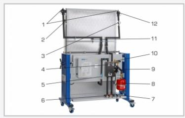
1 vent valves, 2 lighting sensor, 3 flow sensor, 4 thermometer collector outlet, 5 shut-off valve, 6 connectors for warm water, 7 connectors for cold water, 8 diaphragm expansion vessel, 9 circulation pump, 10 pressure relief valve, 11 pressure sensor, 12 temperature sensor
