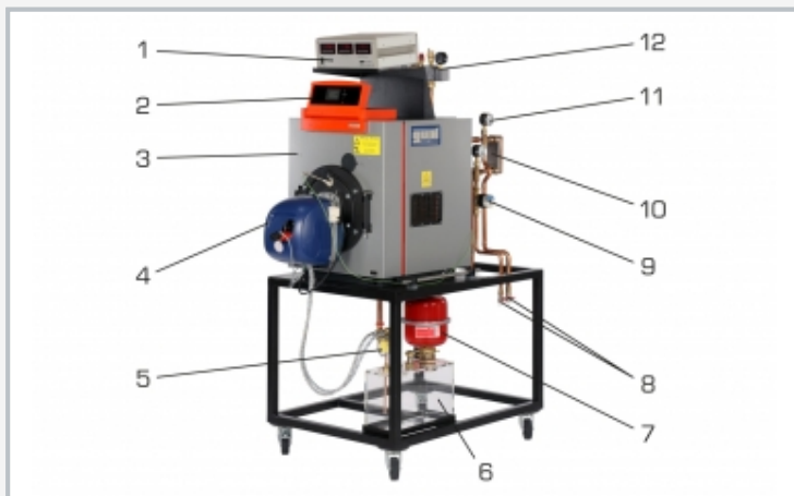
1 measuring amplifier with digital displays, 2 boiler control unit, 3 heating boiler with viewing window, 4 thermocouple, 5 double-strand oil filter, 6 oil tank, 7 expansion vessel, 8 cold water connection, 9 water meter, 10 plate heat exchanger, 11 thermometer, 12 safety group
