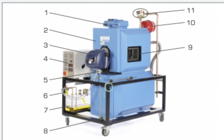
1 heating control unit, 2 heating boiler, 3 HL 352.01 Oil burner [not included], 4 switch cabinet with digital displays and control panel, 5 gas pressure manometer, 6 two-strand oil filter, 7 fuel oil tank with fittings, 8 gas connection, 9 viewing window in the heating control-ler, 10 expansion tank, 11 boiler safety group
