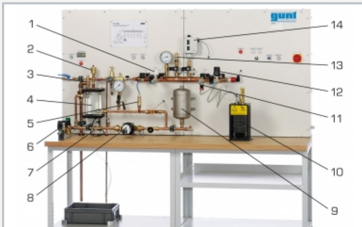
1 thermostatic valve, 2 quick-action ventilating valve, 3 safety valve, 4 air separator, 5 non-return valve, 6 pressure reducing valve, 7 flow switch, 8 pump, 9 expansion vessel, 10 heater, 11 thermal discharge safety device, 12 temperature controller, 13 safety valve, 14 safety pressure cut-out
