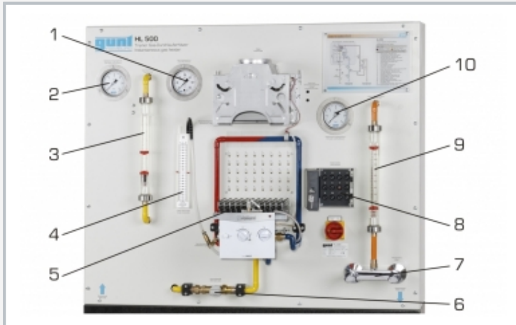
1 gas pressure, 2 water pressure inlet, 3 rotameter for gas, 4 U-tube manometer for differential pressure measurement, 5 instantaneous gas heater, 6 main valve gas, 7 mixer, 8 system faults, 9 rotameter for water, 10 water pressure outlet
