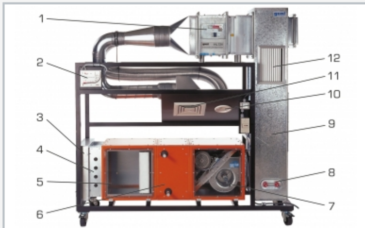
1 fire protection flap, 2 inclined tube manometer, 3 weather louvre, 4 multi-leaf damper, 5 filter, 6 heat exchanger, 7 fan with drive motor, 8 inspection cover, 9 air duct, 10 disc valve, 11 ceiling vent, 12 wall vent
