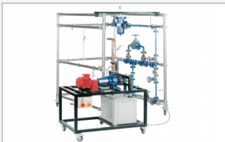
The picture shows HL 960 with a completed specimen installation. In the foreground: pump system HL 960.01.
