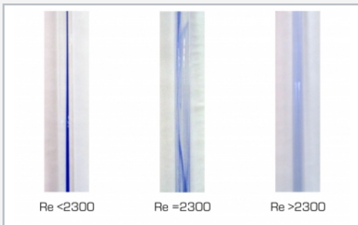
Flow conditions from left to right: laminar flow, transition from laminar to turbulent flow, turbulent flow
