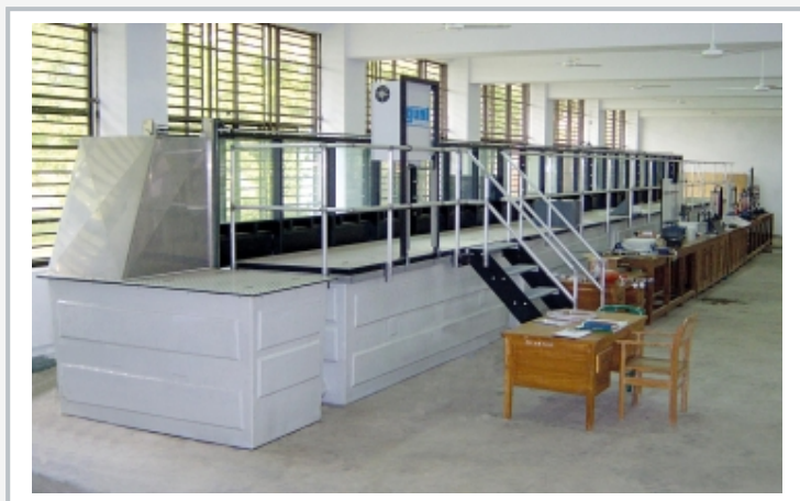
HM 161 with outlet element, gallery and switch cabinet in the foreground.
