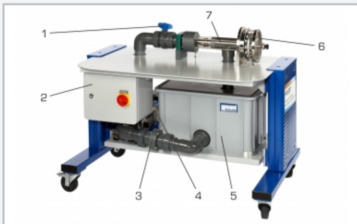
1 valve for adjusting the flow rate, 2 switch cabinet, 3 flow rate measurement with measuring orifice and differential pressure measurement, 4 pump, 5 tank, 6 eddy current brake, 7 axial turbine
