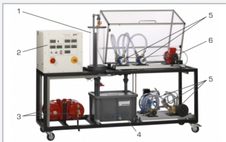
1 measuring tank, 2 displays and controls, 3 stabilisation and pressure vessel, 4 supply tank, 5 pump and compressor models, 6 drive motor
