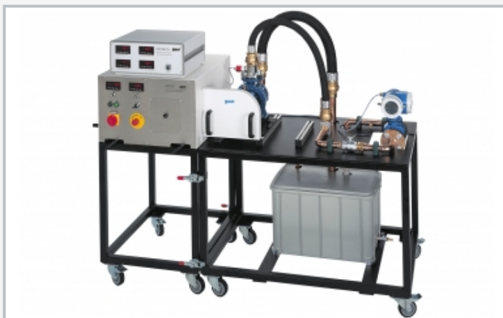
Functional experimental setup: HM 365 drive unit (left), HM 365.10 with pump to be examined (right)
