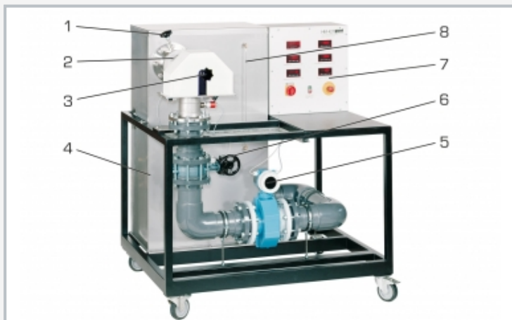
1 lever for adjusting the guide vanes, 2 Kaplan turbine, 3 brake, 4 tank with submersible pump, 5 flow rate sensor, 6 handwheel for throttle valve, 7 switch cabinet, 8 level indicator for tank
