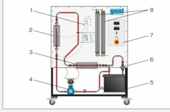
1 differential pressure sensor, 2 vertical measuring location with HM 500.10, 3 horizontal measuring location with empty tube, 4 electromagnetic flow rate sensor, 5 tank with pump, 6 valve to adjust flow rate, 7 switch cabinet, 8 twin tube manometers
