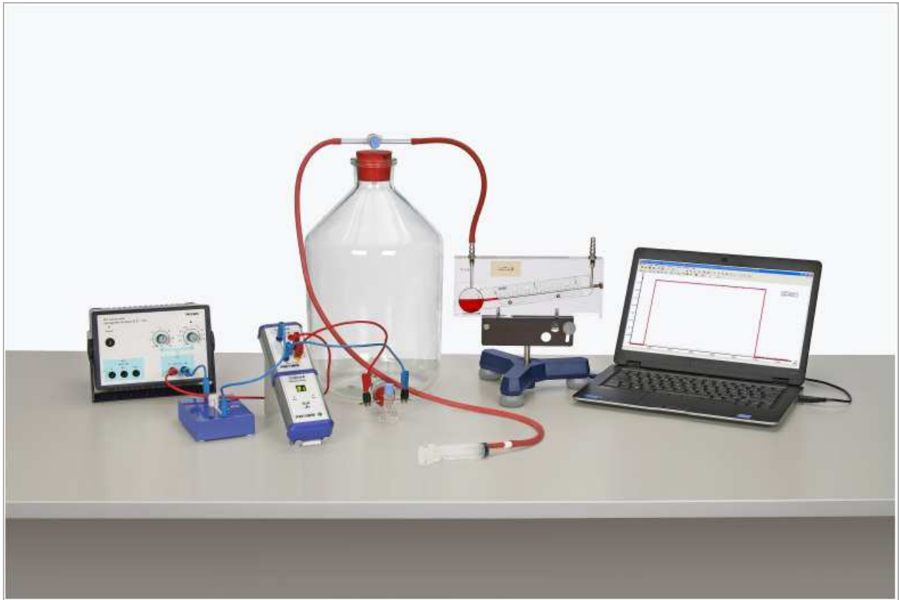
Fig. 3: Experimental set-up for the determination of C_p .
