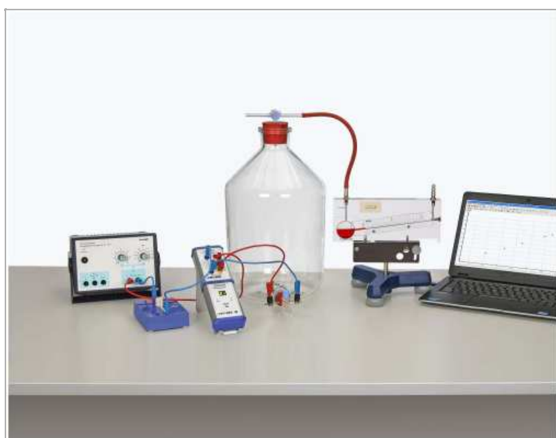
Fig. 1: Experimental set-up for the determination of C_V .
