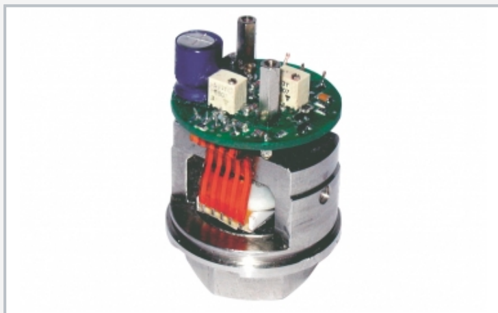
Interior layout of an electronic pressure sensor
