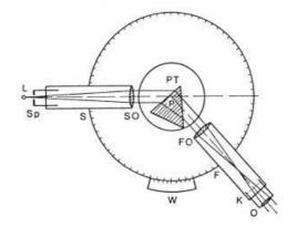
Fig. 2: Set-up and path of rays in the spectrometer. (L = light source, Sp = slit in drawtube, S = collimator, SO = collimator lens, PT = prism table with adjust-ing screws, P = prism, FO = telescope lens, F = telescope, O = eyepiece, K = cross-wires, W = graduated circle with vernier)
