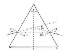
Fig. 5: Refraction by the prism when the path of a ray is symmetrical.
