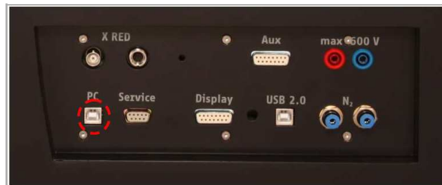
Fig. 4: Connection of the computer
