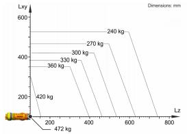
The KR 360 R2830 is designed for a rated payload of 360 kg in order to optimize the dynamic performance of the robot. The maximum payload of 472 kg applies only if the position of the center of mass is 0 mm and a supplementary load optimized for the load case is mounted. The specific load case must be verified using KUKA.Load or KUKA Compose. For further consultation, please contact KUKA Support.
