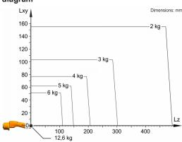
The KR 6 R1840-2 arc HW is designed for a rated payload of 6 kg in order to optimize the dynamic performance of the robot. With reduced load center distances and favorable supplementary loads, a maximum payload of up to 12.6 kg can be mounted. The specific KUKA Load case must be verified using KUKA. For further consultation, please contact KUKA Service.
