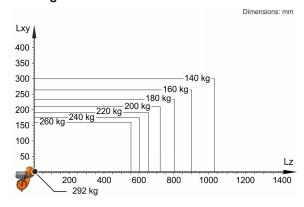
The KR 240 R3200-2 PA is designed for a rated payload of 240 kg in order to optimize the dynamic performance of the robot. With reduced load center distances and favorable supplementary loads, a maximum payload of up to 292 kg can be mounted. The specific KUKA Load case must be verified using KUKA. For further consultation, please contact KUKA Service.
