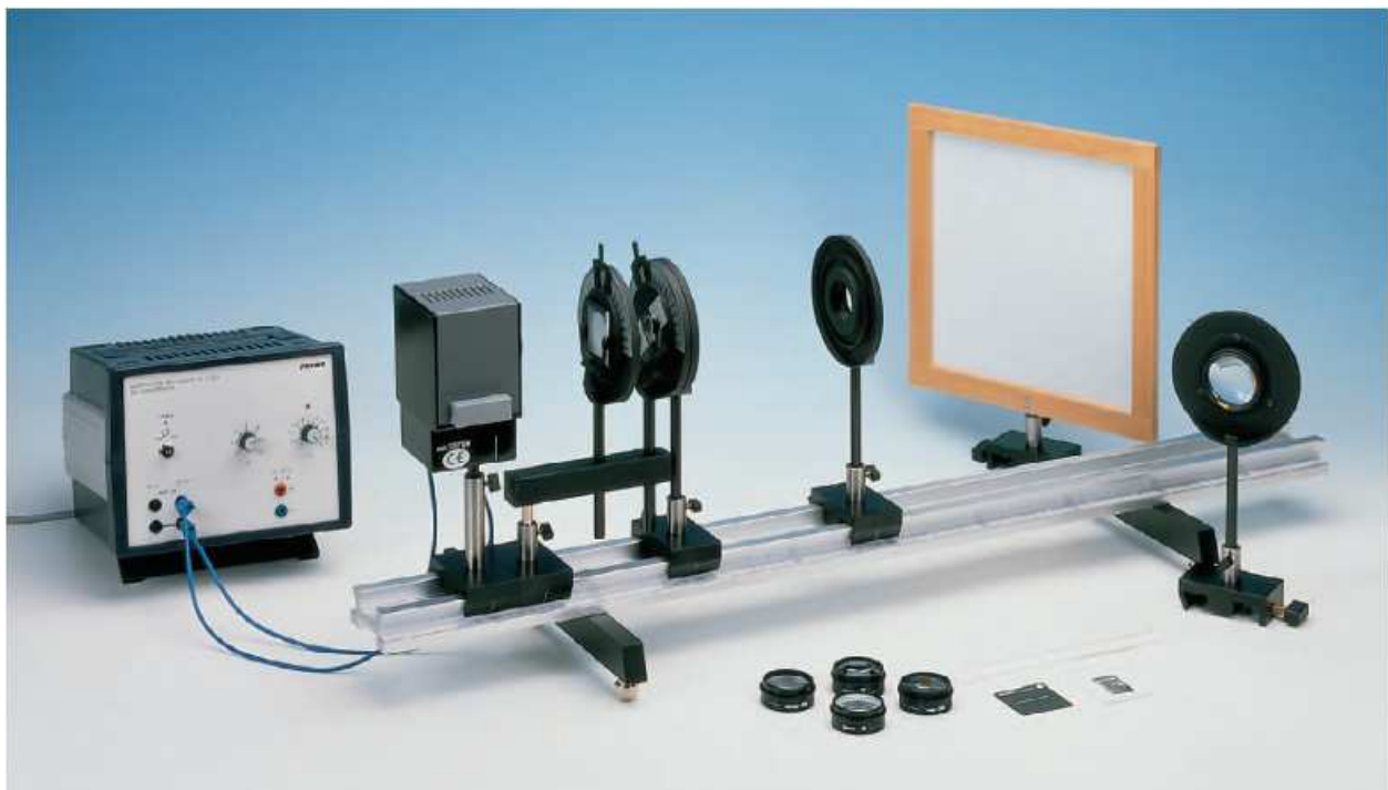
Fig. 1: Experimental set-up (microscope).
