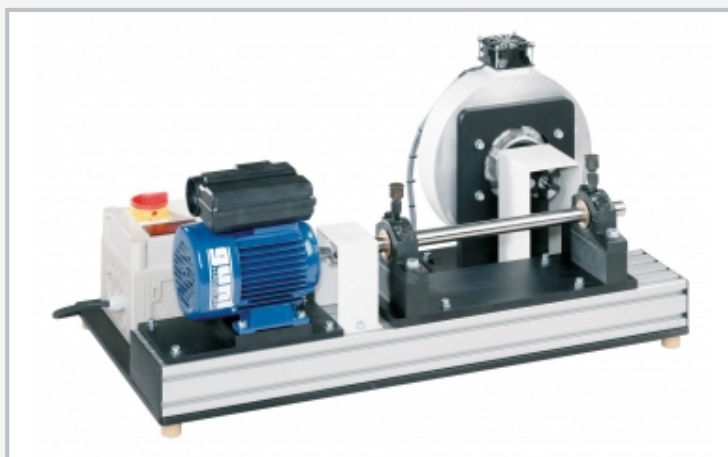
The illustration shows MT 172 together with the journal bearing-mounted shaft MT 170.
