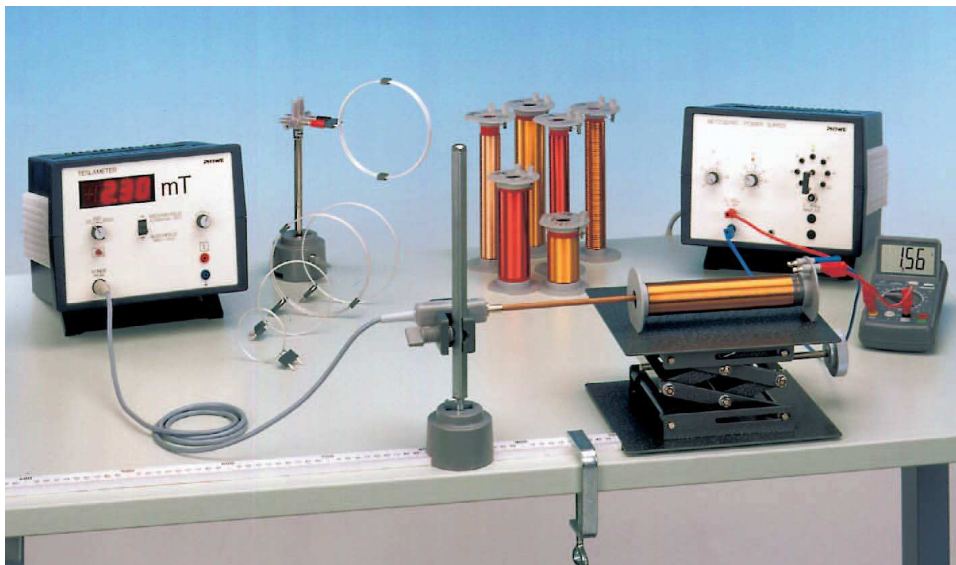
Fig 1: Experimental set-up for measuring a magnetic field.
