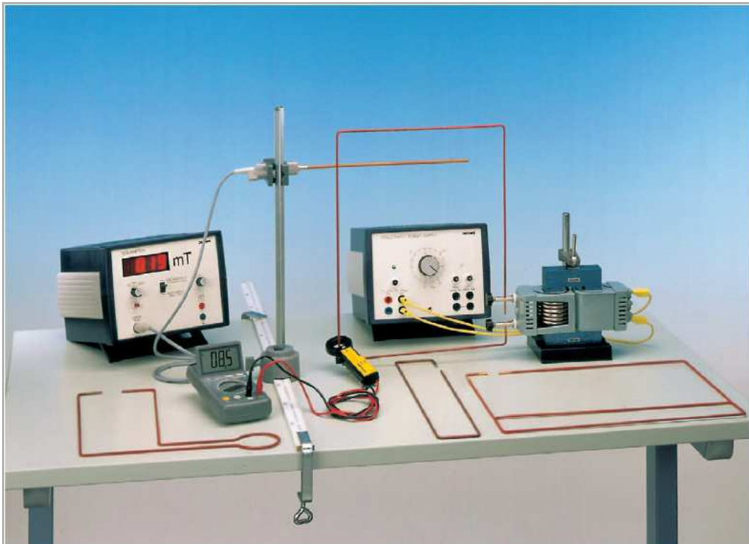
Fig. 1: Experimental set-up for determining the magnetic field in the space outside straight conductors.
