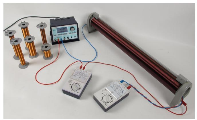
Fig. 1: Experimental set-up with one induction coil slid into the field coil.
