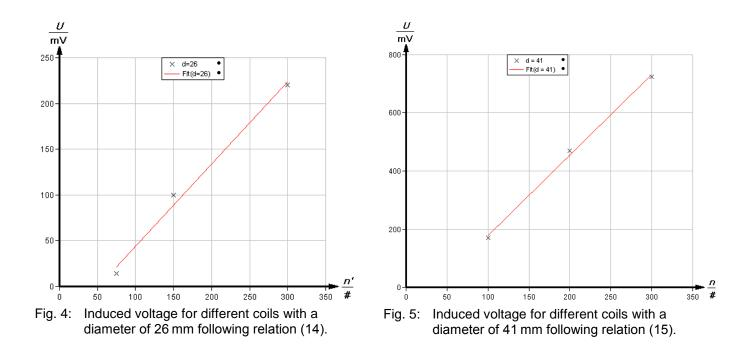
Task 4: Measure the induction voltage as a function of the cross-sectional area of the induction coil at constant frequency and current.
