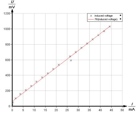
Fig. 2: The graph shows the induced voltage for the coil 11006-01 for varying currents in the field coil. The dependence is linear and follows relation (12).
