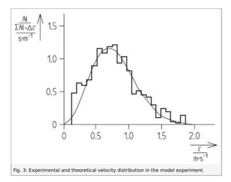
The theoretical distribution function can be evaluated by means of equation (7) using the velocity at the maximum of the experimental distribution as  $c_w$ . The result for the example in Fig. 3 is also shown in the diagram. The agreement between the two curves is reasonably good taking into account the model cha-racter of the experiment.
