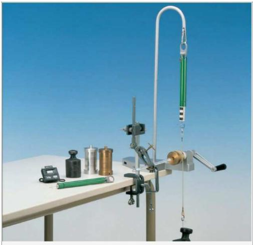
Fig. 1: Experimental set-up: Mechanical equivalent of heat.
