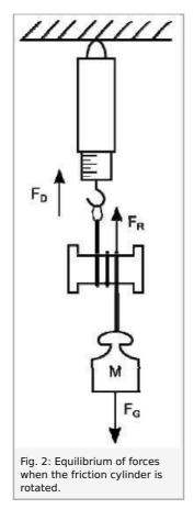
Friction work W is thus determined from the friction path of  $2\pi r\ n$  (r: radius of the cylinder, n: number of turns) and is found to be:
