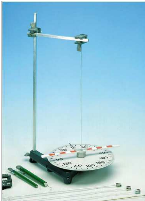
Fig. 1: Experimental set-up for measuring the hysteresis of metal bars in torsion.
