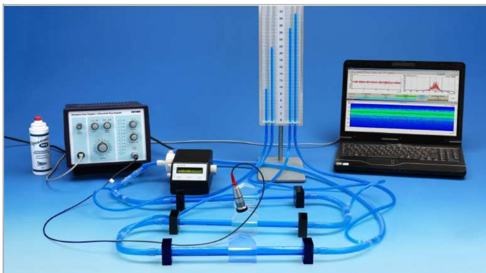
Fig 1: Examination of flowing liquids with Doppler ultrasound techniques, experiment set-up
